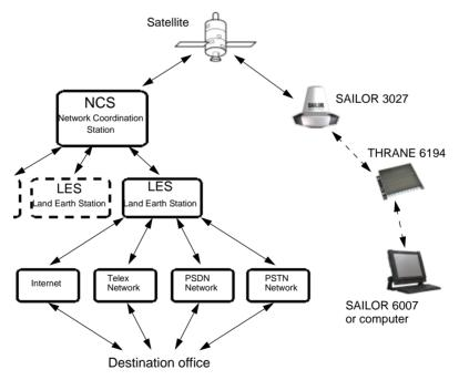
The SAILOR 3027 can work as a standalone system automatically transmitting data on the Inmarsat C network, or you can connect alarm buttons and/or a Message Terminal or a computer through the THRANE 6194 Terminal Control Unit.
